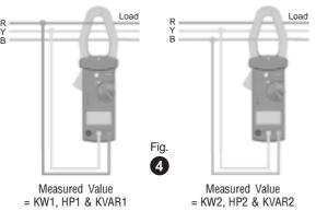
$3\varphi$  Values = (KW1+KW2) or (HP1+HP2) or (KVAR1+KVAR2)  $3\varphi$  PF = Cos[tan<sup>-1</sup>  $\sqrt{3}$ (KW1-KW2) / (KW1+KW2)]
