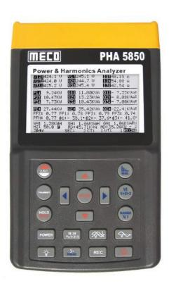
he measurements can be done on Live loads. It is useful in analysing Single—and three-phase quality power systems. It has a large Dot Matrix LCD Display with a Backlight of 35 Parameters on-screen to monitor Energy, Active Power, Apparent Power and reactive Power, Power Factor, Energy, TRMS Value, AC Current, and Average and maximum Demand with Programmable Time Interval and CTR & PTR. It displays Individual Harmonics of Voltage and current up to the 99th Order, THD with Waveform and peak value.
